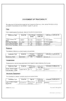
The pressure calibration certificate records the details of the device, a table of measured results and the conditions during the test. The second page displays the reference instrumentation employed during the calibration.
