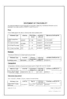
The flow calibration certificate shows the details of the meter, a table of results and the conditions during the test. The second page displays the reference instrumentation employed during the calibration.
