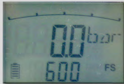
HPM110 showing zero pressure and full scale capability (600 bar)
