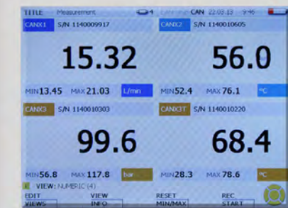
HPM6000 showing two large dials (press down to show additional values)
